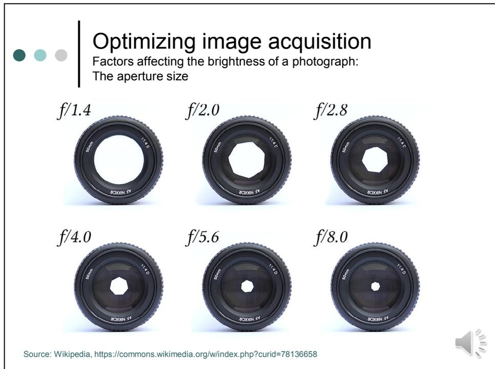
The aperture stop of a photographic lens can be adjusted to control the amount of light reaching the film or image sensor. Typically, a smaller aperture will require longer exposure times to ensure sufficient light exposure. Vice versa, shorter exposure times will require a larger aperture.
