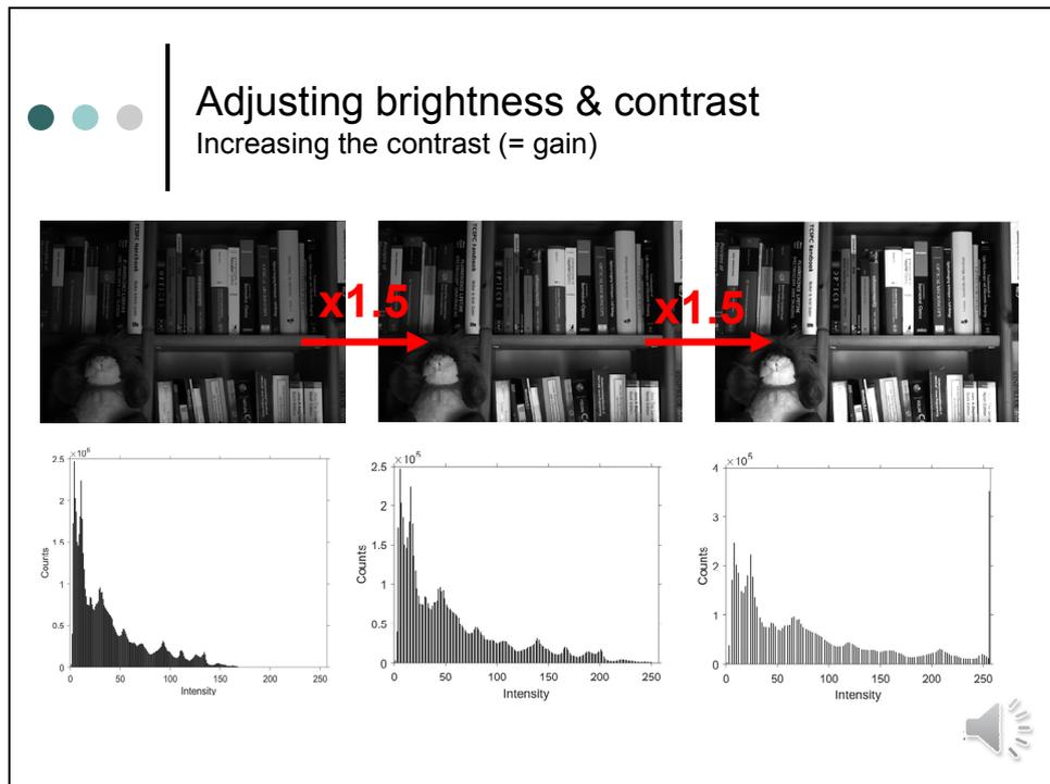
**Contrast** is the difference in brightness that makes an object distinguishable from its surroundings. To increase the contrast between pixels, all what we need to do is to multiply the gray level values of all pixels by some factor. Multiplying the gray level values stretches the histogram. The resulting image becomes brighter and has more contrast.
