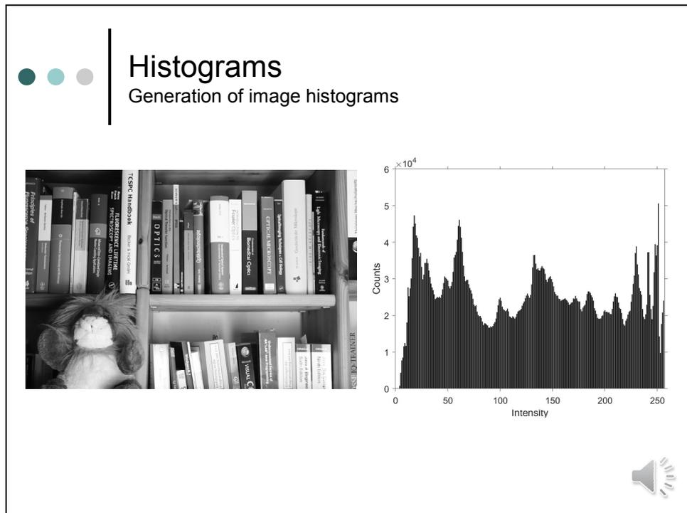
An **image histogram** is a histogram that shows the distribution of gray levels in an image. To create a histogram for a digital image is easy. The bins represent the gray levels, and the x-axis spans the entire bit range of an image.
