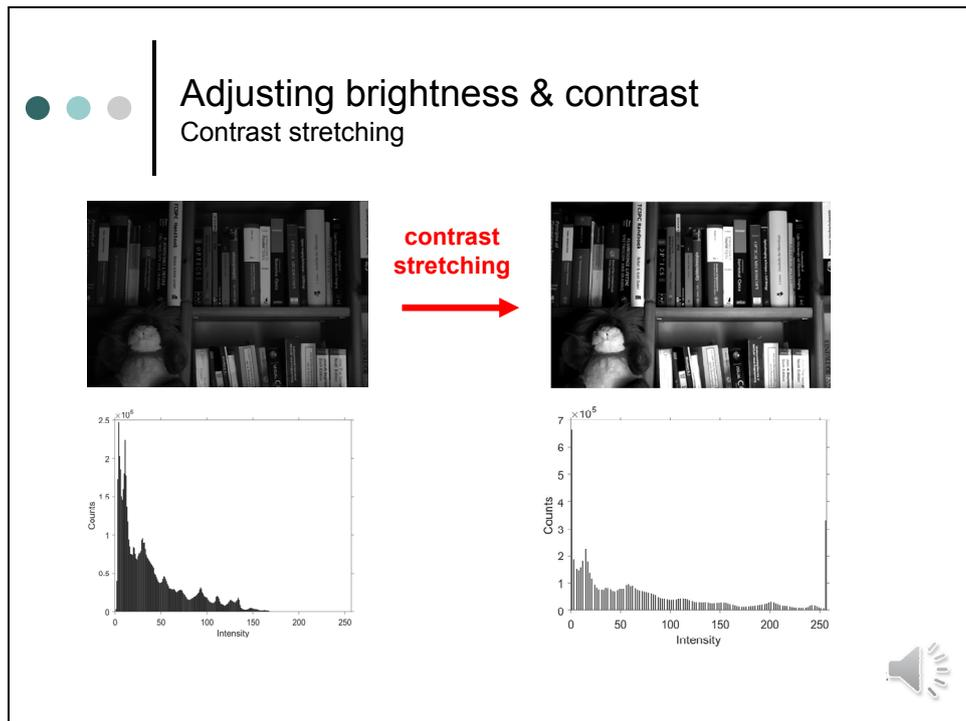
This slide shows the result for the contrast stretching operation applied to our test image. Here, the lowest and highest input value have been chosen such that in the transformed image ~5% of the pixels are saturated at zero and ~5% of the pixels are saturated at 255.
