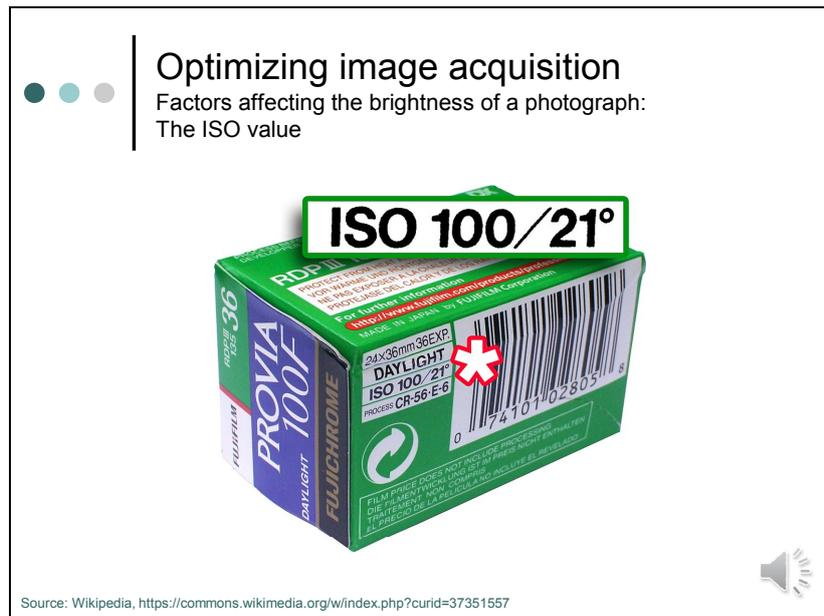
In analog photography the iso value specifies the sensitivity of a photographic film to light. The value is also referred to as film speed. A relatively insensitive film, requires long exposure to light and is thus termed a *slow film*. Highly sensitive films can achieve the same result with shorter exposure times and are correspondingly termed *fast films*. To quantify the film speed several standards are used.
