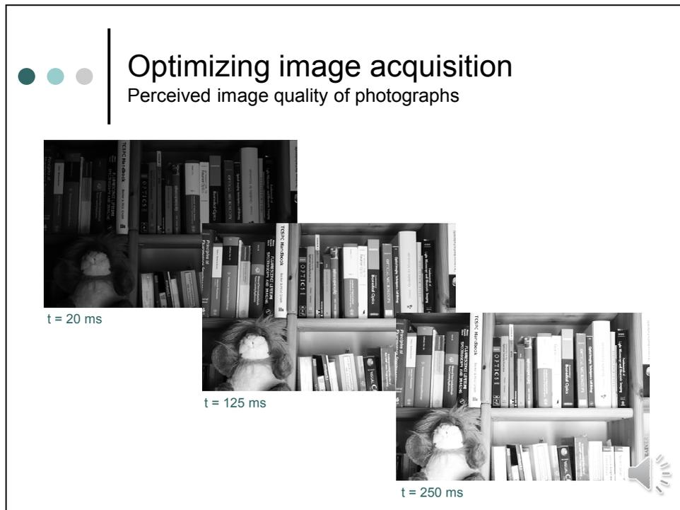
This slide gives an example, about how image histograms can be used to assess the image quality. In the series of images which you can see here, only the exposure time has been varied.
