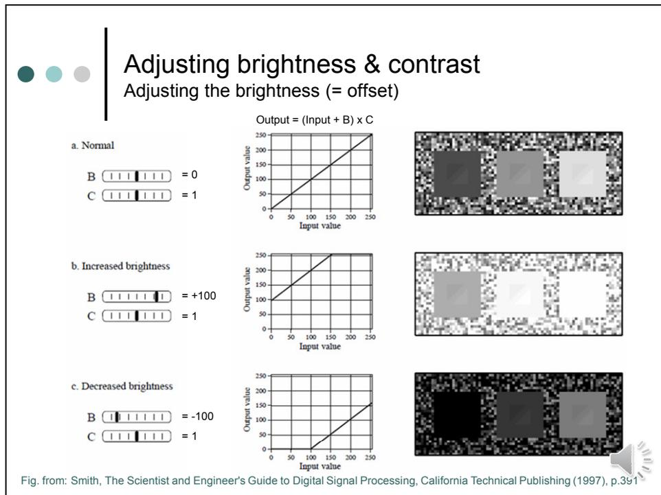
A) In the first example brightness and contrast are set at the *normal* level, as indicated by the **B and C slide bars** at the left side of the image. This means brightness (i.e. the offset) is at 0 and contrast (i.e. gain) is 1. Under these conditions the intensity transform function does nothing. Output values for display equal the input values.
