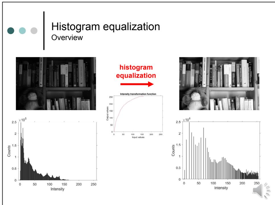
All what we have to do, is to calculate the cumulative histogram and scale it to the bit range. This yields the intensity transform function for histogram equalization. When we now use this look up table, we get the contrast enhanced picture. The improvement is evident.
