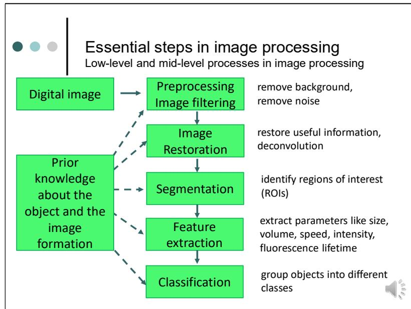
The first steps in image processing are low-level processes: Input and output are images.
